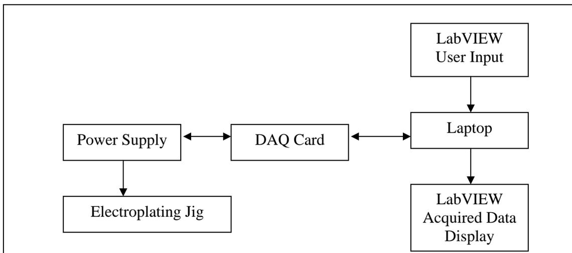
**Figure 5 : Illustration of Electroplating Setup**
