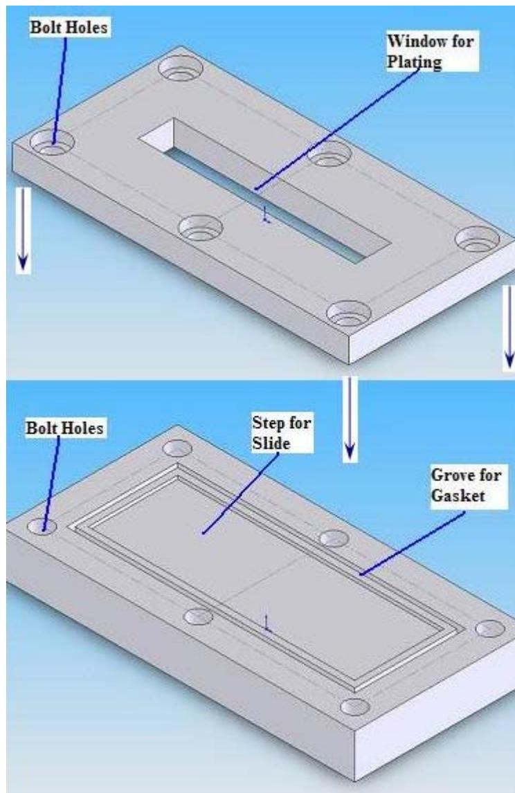
**Figure 3 : Assembly Diagram for Square Jig**
