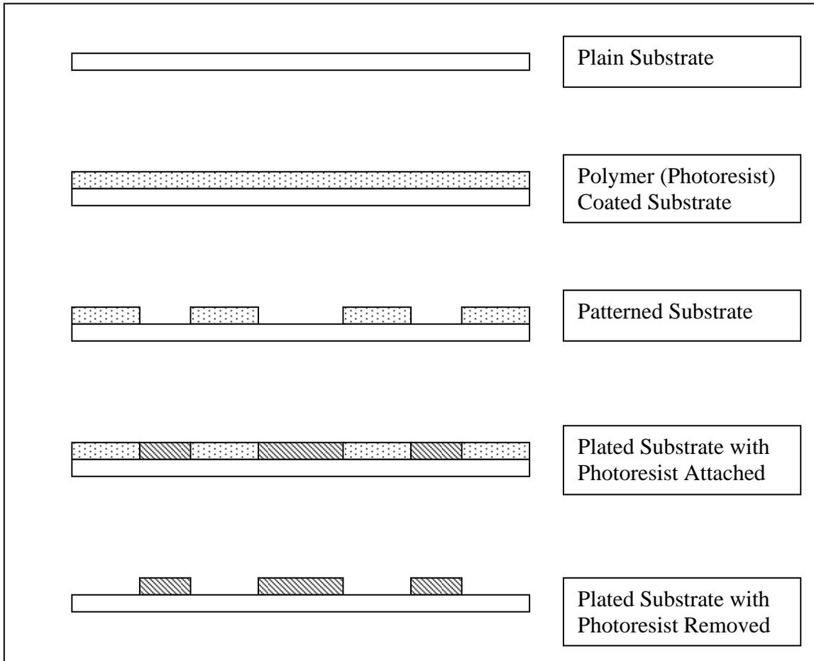
**Figure 6 : Schematic of Substrate Processing**
