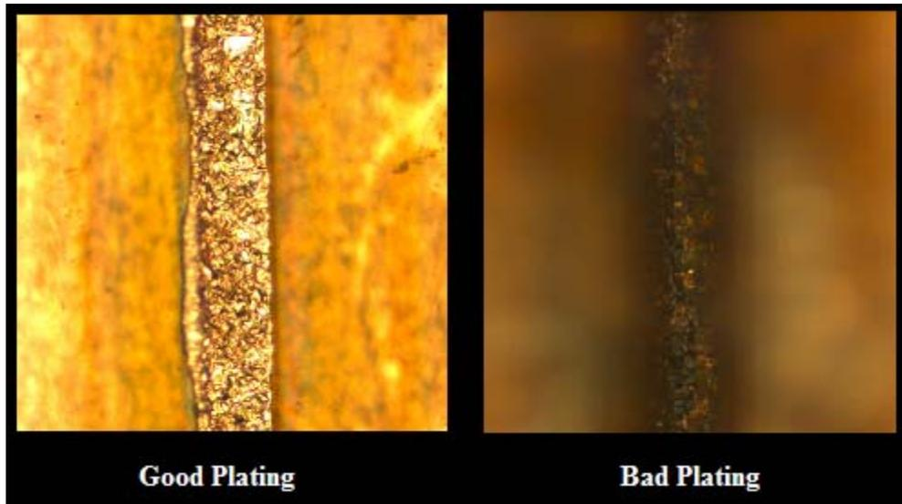
**Figure 20 : Comparison of Bad Plating & Good Plating**
