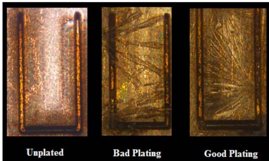
**Figure 19 : Comparison of Bad Plating & Good Plating**
