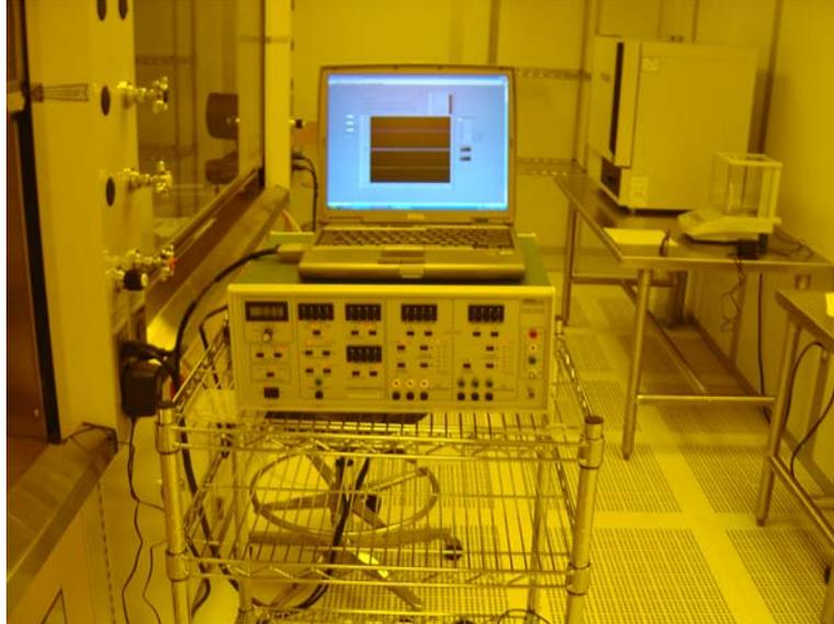
**Figure 12 : Laptop with LabVIEW Interface Attached to Power Supply**
