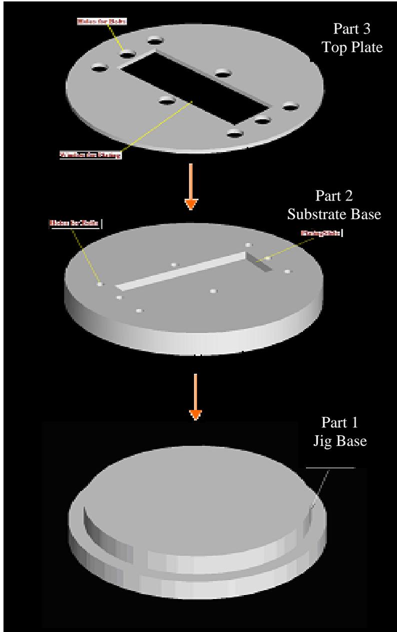
**Figure 1 : Jig Assembly Diagram**
