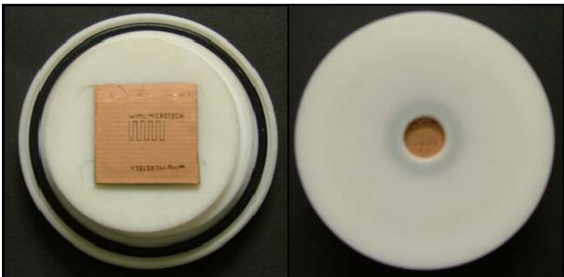
**Figure 16 : 1 x 1 inch Adapter Plate & Sample**
