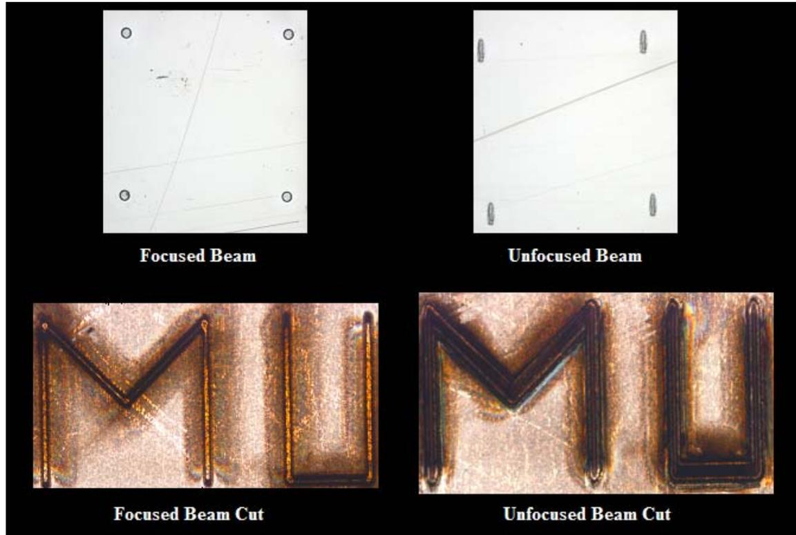
**Figure 7 : Patterns of Unfocused vs. Focused Beam Cuts**
