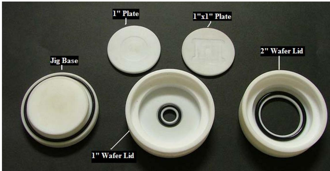
Figure 14 : Elements of the Circular Jig
