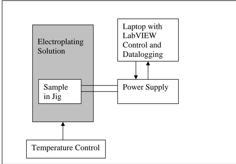
**Figure 11 : Block Diagram of Electroplating Setup**
