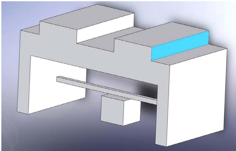
Figure 11: This design was very compliant in the z-direction but was not stiff enough in the x-direction (cutting direction). This would cause vibration of the tool and a rotational motion of the beam can cause the tool to wear away from the cutting edge radius.
