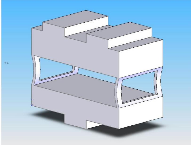
Figure 10: The wall thickness from Figure 9 was increased to 2mm. This yielded in a total deflection of 2.5mm and significantly reduced the buckling of the frame.
