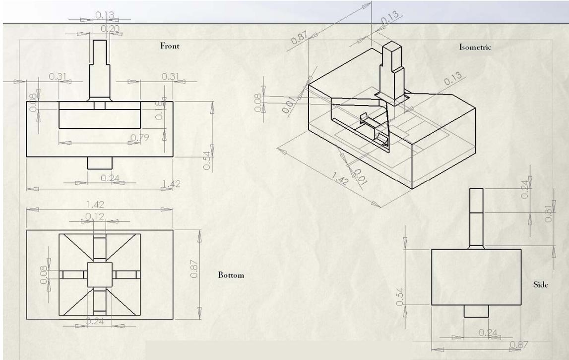
Figure 14: Shows the e-drawing of four different views of the final compliant suspension design with their corresponding dimensions in inches.
