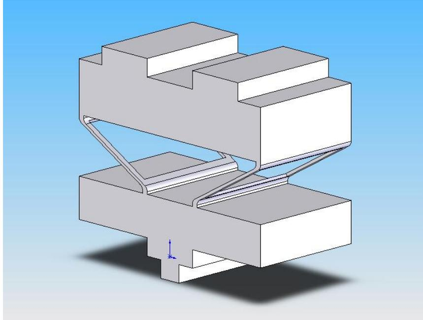
Figure 8: The edges from Figure 7 were rounded to make the system more compliant. The idea worked but the deflection was still insufficient ( $\approx 500\mu\text{m}$ ).
