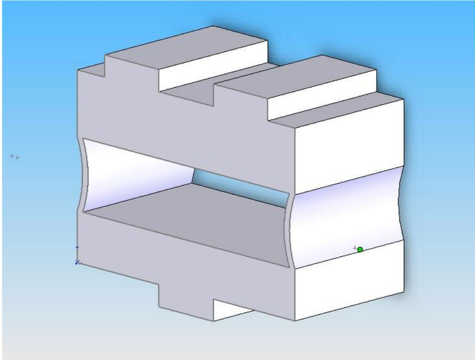
Figure 3: A compliant design with a 1mm thick arched wall that would act as a spring mechanism.
