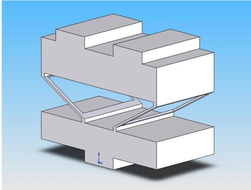
Figure 6: This is basically an improvisation of Figure 5 where now only a frame is along the sides. This means lesser material and technically more deflection. The idea worked but the deflection was still not sufficient ( $\approx 400\mu\text{m}$ ).
