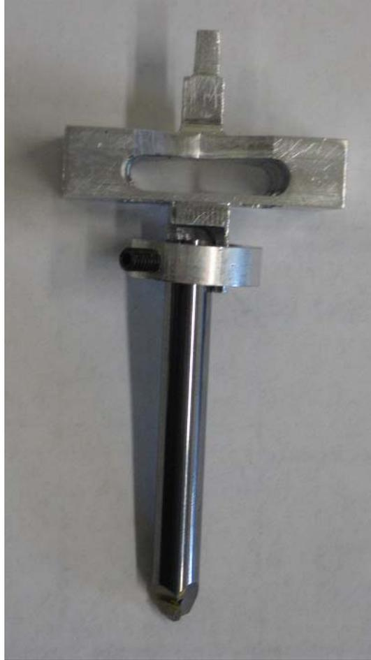
Figure 19: Image shows a diamond tool clamped on the compliant suspension with a collar.
