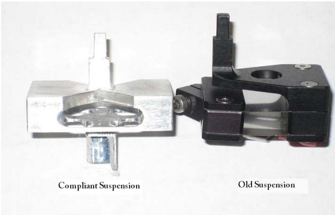
Figure 21: Image compares the new compliant suspension and the old suspension by CETR. The new suspension is slightly more compact in size.
