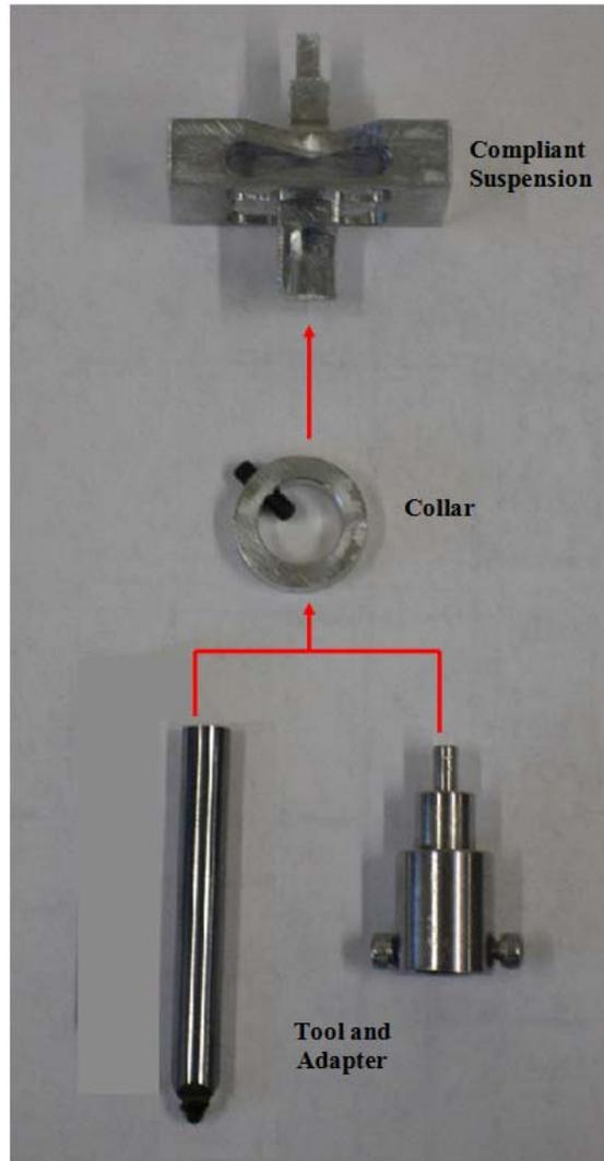
Figure 18: The image shows the assembly diagram for the compliant suspension.
