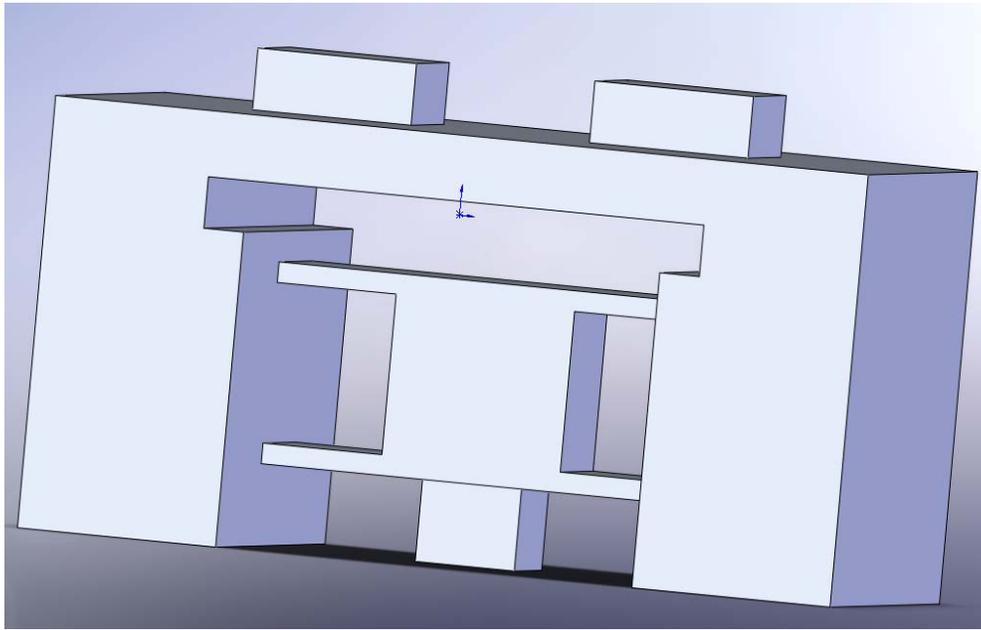
Figure 12: The design was not compliant enough in the z-direction. It only yielded a maximum deflection of  $20\mu\text{m}$  for a load of  $1700\text{mN}$ . If the compliant sections were to be any thinner than the above shown, this would yield in rotation in the x-axis causing the tool to vibrate.
