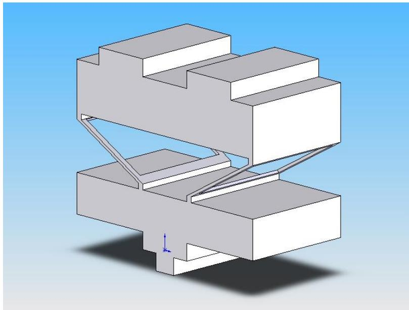
Figure 7: Very similar to Figure 6 except that the extra section was added at the bottom to act as the tool area.
