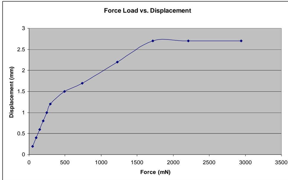
Figure 2: Displacement versus force-load ratio used to design the suspension
