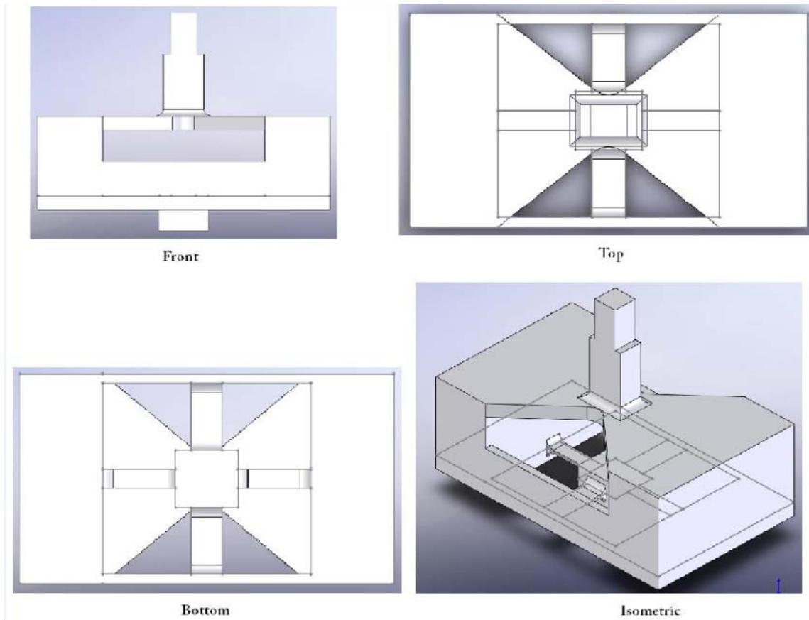
Figure 13: Shows the CAD drawing of four different views of the final compliant suspension design.
