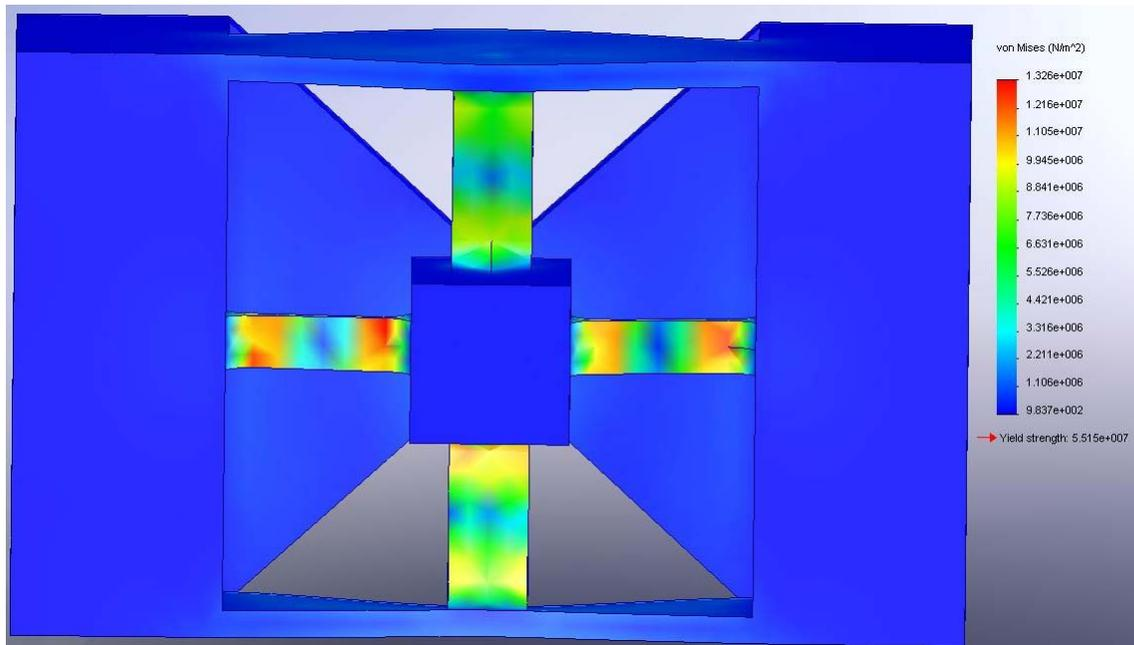
Figure 17: FEA showing the von Mises stress distribution in the compliant section of the new suspension.
