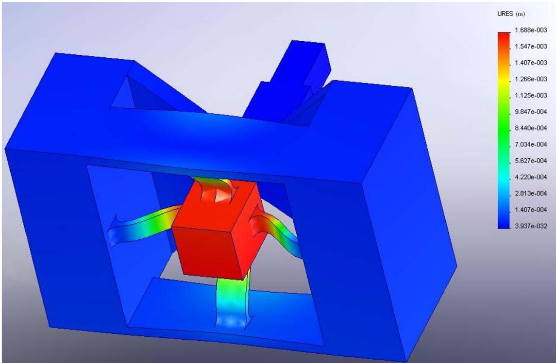
Figure 16: FEA showing the deflection in the compliant section of the suspension.
