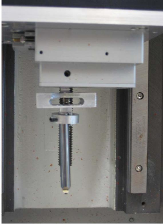
Figure 20: Image shows the suspension in the load cell on the UMT.
